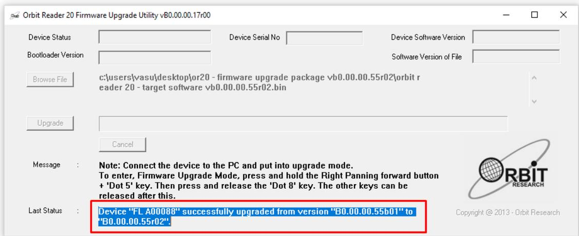
13. The Orbit Reader is upgraded. Turn on the Orbit Reader to start using the device.
