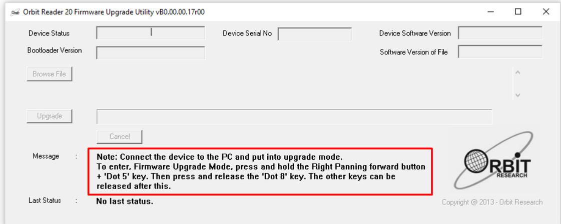
4. Press and hold down the Right Panning forward button + Dot 5, then press Dot 8. The utility shows the message “Orbit Reader 20 is connected” in the device status field. It shows the message “Do you want to upgrade the device?” in the message field at the bottom of the dialog.
