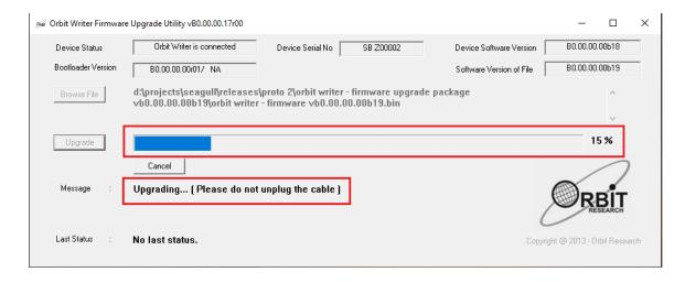
12. Do not unplug the cable. Wait for the message "Device upgrade has been completed" on the upgrade utility or until the Orbit Writer reboots and shuts down.
